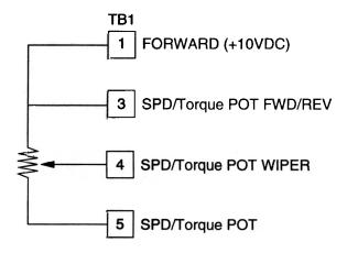
External analog voltage input example:
