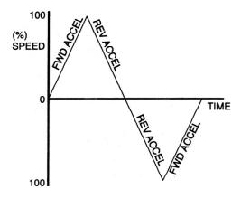
The FWD and REV ACCEL trimpots are factory adjusted to 3.5 sec. The acceleration times are adjustable to a maximum of 8 seconds.
