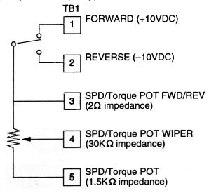
Bidirectional (without switch) operation example: Directional changes of the motor shaft in speed or torque operations is accomplished by adjusting the potentiometer. (The Min. pot can not be used).
